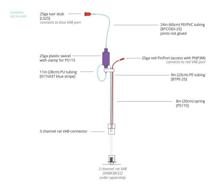
Dead Volumes Blue channel: 135μL Red channel: 40μL White channel: not connected (±15%, not including button or catheter)
