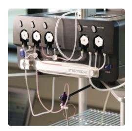
Add Instech's Automated Blood Sampler to a tethered animal and it will take the blood samples for you at your programmed time points and store them in a refrigerated fraction collector.
