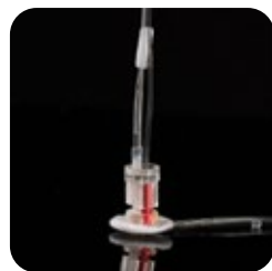
The specially designed glucose-clamp tether has one line for blood sampling and a second for infusion, with a built-in Y connector close to the animal for tracer injection. The lightweight looped wire keeps lines organized and turns the swivel.
