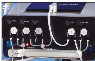
Instech uses five P625/66 pumps in its automated blood sampler for laboratory animal research
