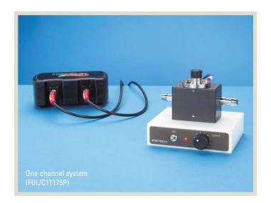
his system is based on a fiber optic fluorscence lifetime measurement of oxygen concentration, the most advanced, efficient and stable technique available. The system reads the oxygen concentration in the medium surrounding the test specimen and, when sealed, yields a accurate measure of the oxygen consumption rate (OCR).
